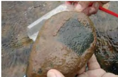
Step 6. The scraped area is rinsed with water until the cut-out area is completely clear.
