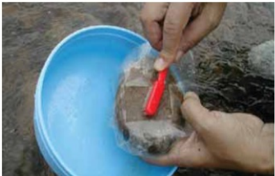
Step 5. Benthic diatoms on the surface of the selected stone are brushed off.
