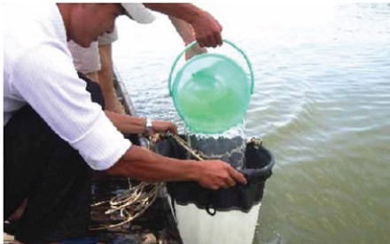
Step 2. Collect 10L of water and filter it slowly through the plankton net.
