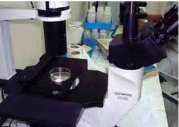
Step 4. Transfer the sample to a Petri dish and examine it under a stereo-microscope at a magnification of 40x to identify the larger specimens of zooplankton.
