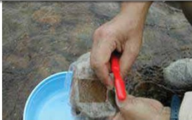
Step 4. A plastic sheet with a 10 cm 2 cut-out is placed on the upper surface of the selected stone.
