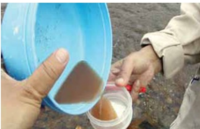
Step 7. Each sample is poured into a plastic bowl and then into a plastic container.
