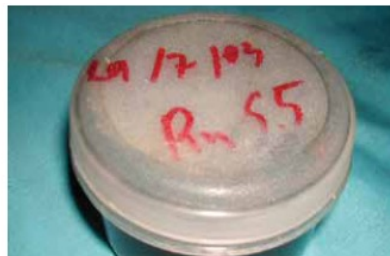
Step 8. The label includes the site name, the site code, the date, and the replicate number, written on the plastic container.
