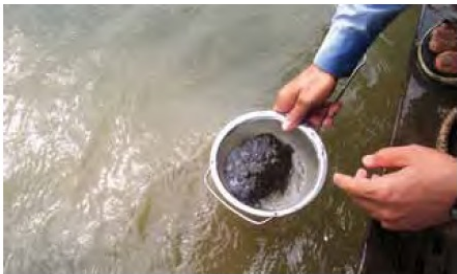
Step 5. Remove some of the sample and place it in a smaller-sized sieve with a 0.3mm mesh for further washing.
