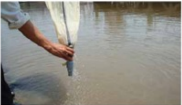
Step 4. Rinse the bottom of the net to result in a water volume of about 150mL.
