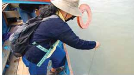
Light penetration is recorded by slowly lowering the Secchi disk into the water until it just disappears
