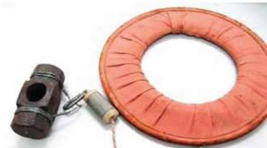
Water depth determined by dropping a weighted rope directly to the river bottom
