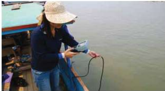
Temperature, DO, pH, EC are recorded using an electrical metre
