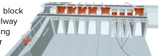
Figure 3-5 The spillway structures including the surface and Low-Level Outlets. View is from upstream
